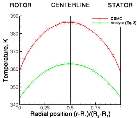
Figure 3. Temperature profiles at 10 Pa (Test #7).
