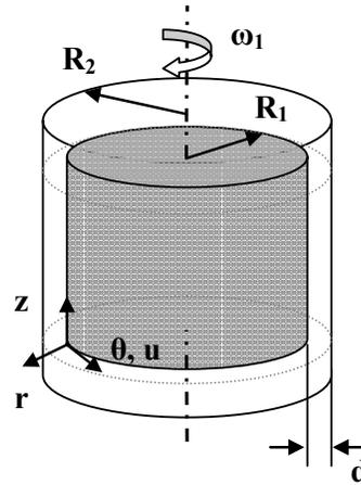
Figure 1. Flywheel schematic with stretched scale for clarity.
