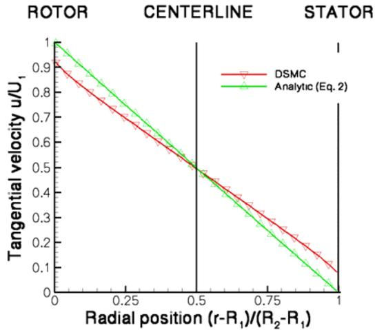
Figure 4. Velocity profile at 10 Pa (Test #7).
