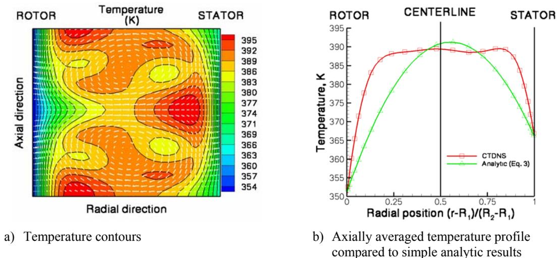
**Figure 7. Temperature contours in the  $(r, z)$  plane and accompanying  $(v, w)$  velocity vectors (left) and axially averaged temperature profile (right) (Test #6).**
