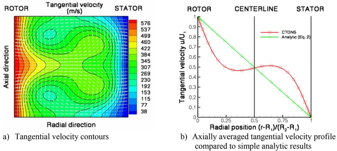
**Figure 6. Tangential velocity contours in the  $(r, z)$  plane and accompanying  $(v, w)$  velocity vectors (left) and axially averaged tangential velocity profile (right) (Test #6).**
