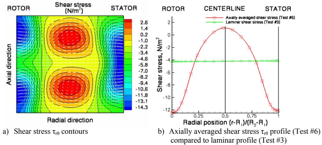
**Figure 8. Shear stress  $\tau_{r0}$  contours in the  $(r, z)$  plane and accompanying  $(v, w)$  velocity vectors (left) and axially averaged shear stress  $\tau_{r0}$  profile (right) (Test #6).**
