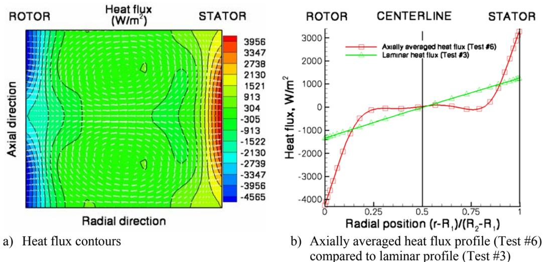
**Figure 9. Radial heat flux contours in the  $(r, z)$  plane and accompanying  $(v, w)$  velocity vectors (left) and axially averaged radial heat flux profile (right) (Test #6).**
