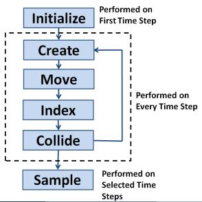
DSMC collisions are performed statistically. Pairs of molecules are randomly selected from within a cell, a collision probability is calculated for each selected pair, and a random number draw determines whether or not the pair actually collides.
