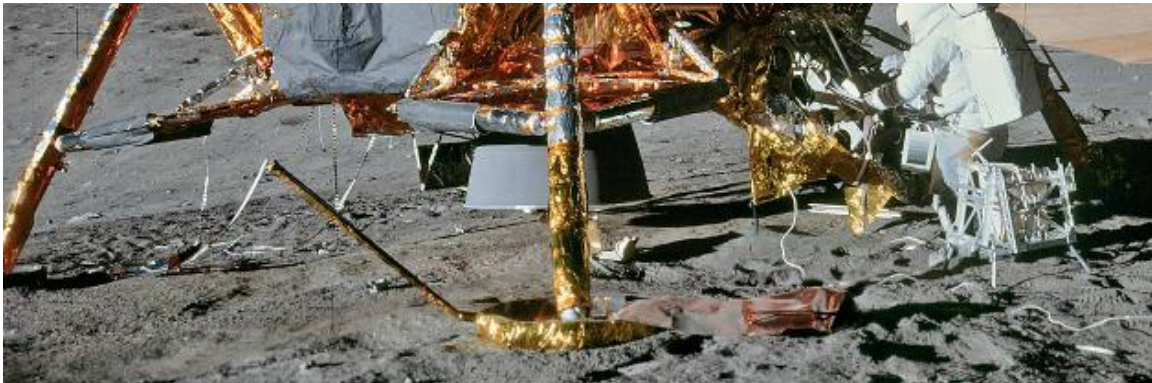
Figure 2.4.1. View underneath the Apollo 12 Lunar Module showing that cratering does not occur and that viscous erosion is the likely dominant scouring mechanism.
